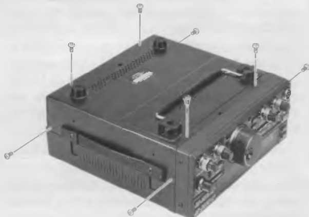
Figure 1: Bottom Cover Removal
