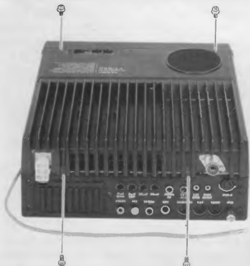
Figure 5: Local Unit Shield Cover
